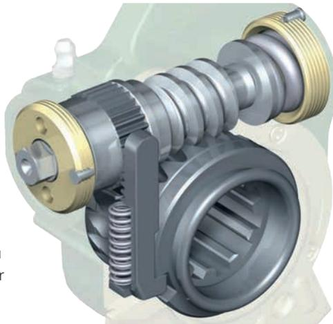
Once the mechanism has been 'de-adjusted', a ring spanner on the hex end will show whether it comes back into adjustment: the spanner should rotate further clockwise each time the brake pedal is applied and released, until adjustment stops. Finally, the brake needs to be 'reset', according to the specific instructions from the manufacturer.
